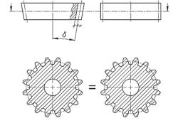
Fig. 1. Comparison of Beveloid gear geometry with a spur gear
