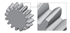
Fig. 2. The shape of the tooth space in Beveloid gear
