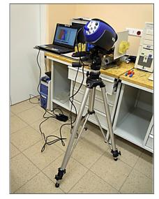
Fig. 8. Thermal imaging camera type FLIR SC5000
