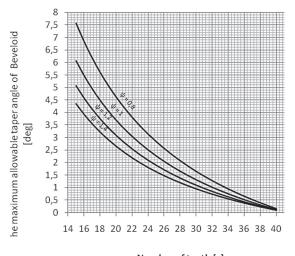
Number of teeth [z] Fig. 6. Maximum allowable narrowing angle in Beveloid gears [deg]
