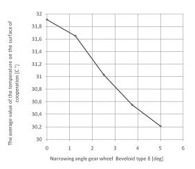
Fig. 12. The results of measurements, for the various gears, measured as the average surface temperature of gear mate
